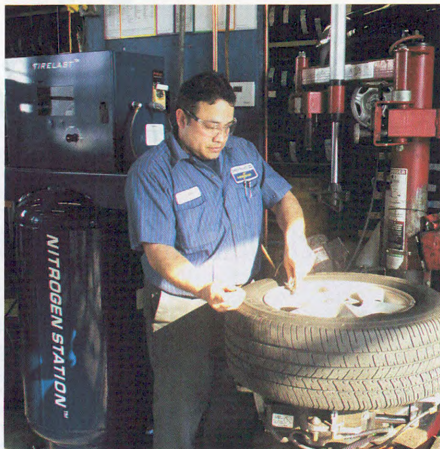
Craven Tire & Auto tech Jesus Toledo installs nitrogen at one of the dealership's shops. "We put nitrogen in everything now," says Craven Tire President Steve Craven. The company offers nitrogen at all of its stores.
